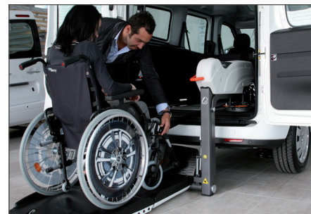
Front tie down of the wheelchair is made before lifting it up, maximizing comfort for the caregiver and safety for the wheelchair user
