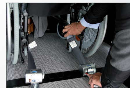
The Fiorella Lift equipped with F-Twister option eases rear access to the vehicle, in order to perform rear tie-down from a comfortable and safe position.
