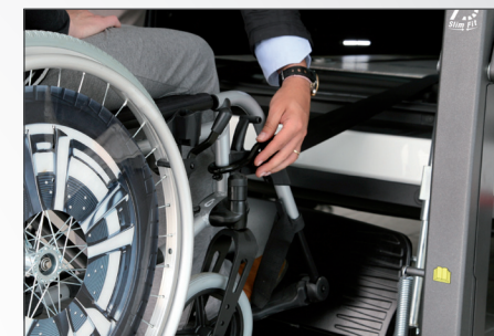
Front tie down of the wheelchair is made before lifting it up, maximizing comfort for the caregiver and safety for the wheelchair user
