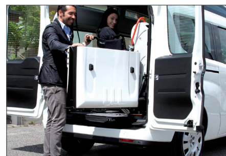
The Fiorella Lift equipped with F-Twister option eases rear access to the vehicle, in order to perform rear tie-down from a comfortable and safe position.
